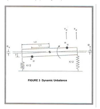
http://www.BetaMachinery.com the dynamic unbalance mass, md rotating at a radius, r and speed, w
