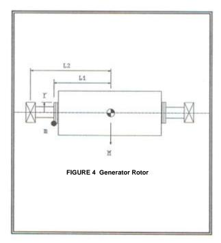
Total rotor mass: M = 11,800 kg Operating Speed: w = 3600 rpm  $1^{st}$  Critical Speed: w<sub>c</sub> = 1350 rpm Radius for Balance Weights: r = 14" L<sub>1</sub>/L<sub>2</sub> ratio: c = 0.67
